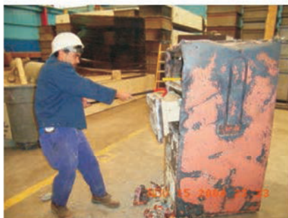
Actual Tests conducted on the Godrej FRFC at Underwriters Laboratory, USA for Fire Endurance, Fire & Impact (which includes the unique 9 metre drop test) and Explosion Hazard Test.
